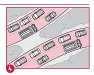
Provide two or more suitably sized access and egress routes to accommodate the movement of emergency vehicles.
