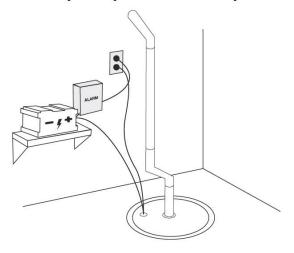
Sump pump failure is a leading cause of basement flooding. Check your SP each season to ensure it's functioning properly. Install/maintain a backup battery to keep it functioning in the event of a power outage. Visit <a href="www.homefloodprotect.ca">www.homefloodprotect.ca</a> for more flood prevention tips.
