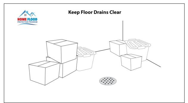
A blocked floor drain will prevent water from exiting your basement during a flooding event. Remove any items that are blocking the flow of water to your floor drain. Remove debris from the drain as needed. Visit <a href="www.homefloodprotect.ca">www.homefloodprotect.ca</a> for more flood prevention tips.
