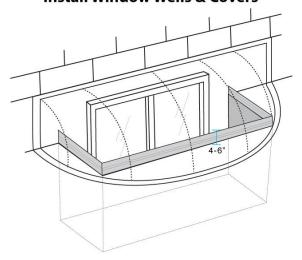
Water that pools against your windows can make its way into your basement. Install window wells that sit 4-6" above ground and are sealed at foundation. Consider installing window covers to further reduce risk. Visit <a href="https://www.homefloodprotect.ca">www.homefloodprotect.ca</a> for more flood prevention tips.
