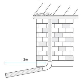
Clogged eaves troughs and short downspouts can cause water to collect at your foundation and seep into your basement. Remove debris and extend downspouts at least 2m from foundation onto a permeable surface. Visit <a href="https://www.homefloodprotect.ca">www.homefloodprotect.ca</a> for more flood prevention tips.
