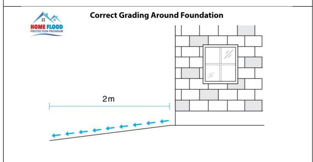
Poor grading can direct water into your basement through foundation cracks and damaged window seals. Correct grading to ensure that water flows at least 2m from foundation, or towards a drainage swale. Visit <a href="www.homefloodprotect.ca">www.homefloodprotect.ca</a> for more flood prevention resources.
