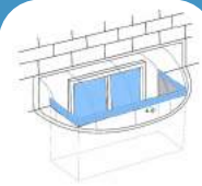
Install Window Wells that Sit 10-15 cm Above Ground and Upgrade to Water Resistant Windows
