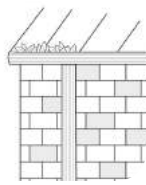
Clean Out Eaves Troughs
