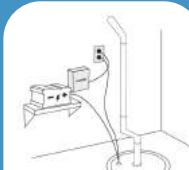
Install Backup Sump Pump and Battery
